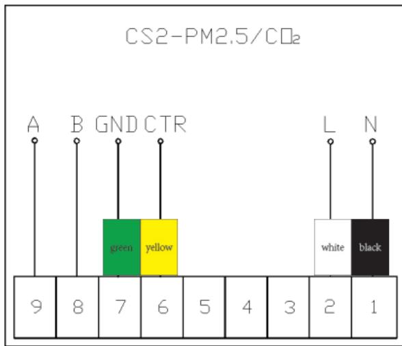
(According to the color wiring shown in the figure, the equipment wiring corresponds to it one by one.)
